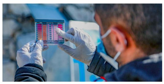
A water and sanitation staff is measuring the clarity of the water. The percentage of chlorine is measured to make sure it is safe for human consumption. © Syria Relief
