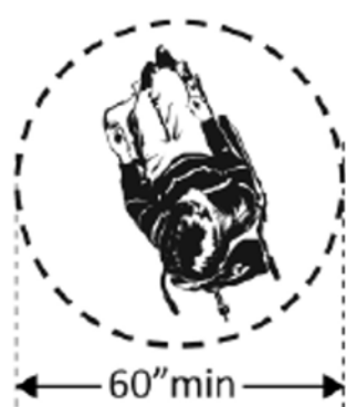
Figure C1_2.1_1: Circular turning space
