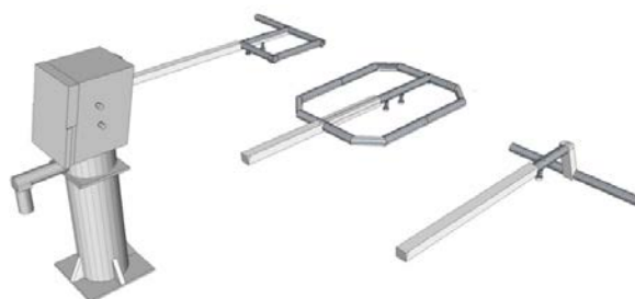
Figure C2_9.3_1: Example of pump handles
