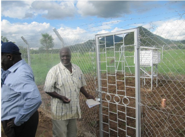
Kapedo Health Centre 3 weather station constructed by World Vision IMTAC funds with Stevenson screen and rain gauge enclosed in chain link (Kaabong District)
